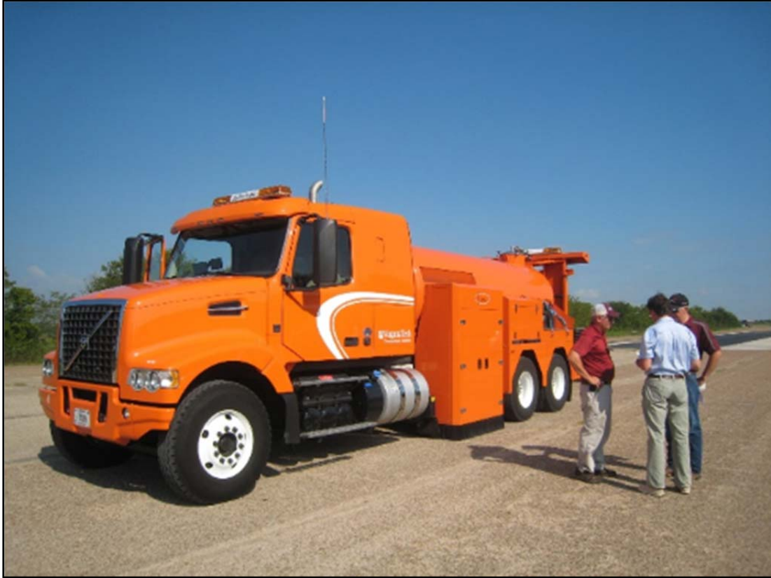
Figure 7. SCRIM Continuous Friction Measurement Equipment.
