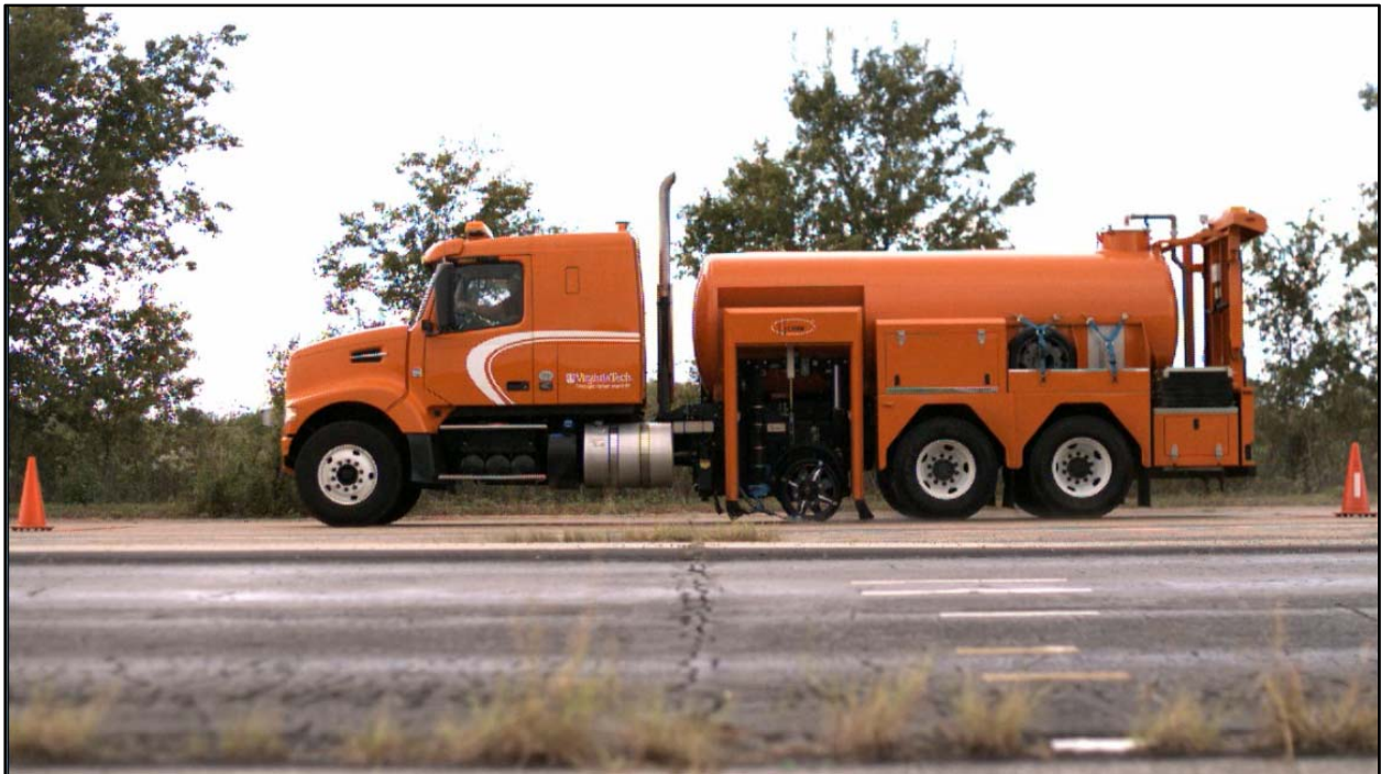
Figure 17. SCRIM Percent Slip Verification Test Setup.
