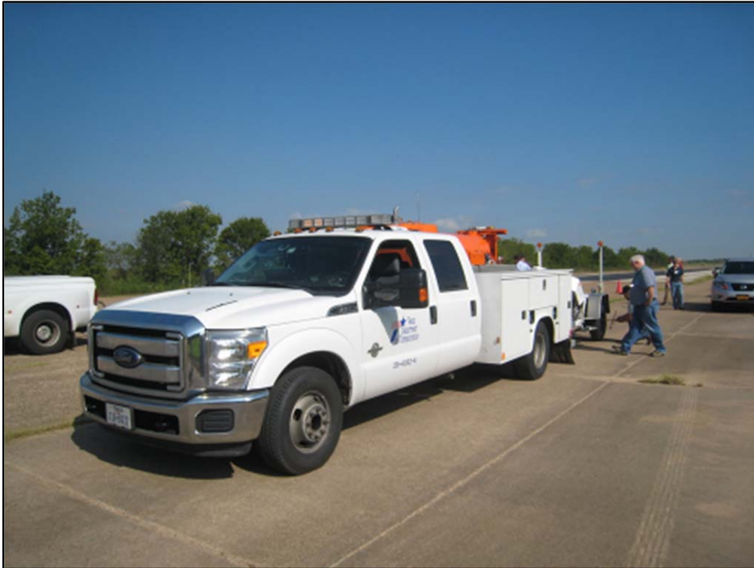
Figure 9. TxDOT Locked-Wheel Skid Trailer (29-4382K).
